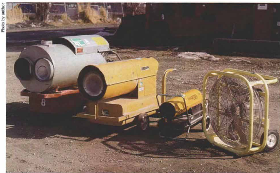
Portable space heaters and fans are a big help in cold weather. From left to right is a 500,000 Btu vented heater, a 320,000 Btu unvented heater, a 100,000 Btu unvented heater and a 30-in. hot-air balloon fan for inflating temporary polyethylene air structures. Vented space heaters are the best choice for curing concrete and for heating enclosures with people inside, while unvented heaters are great for warming up building materials and tools.
